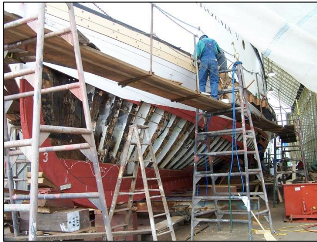
Hull planking being replaced during the vessel's dry-docking in 2005
