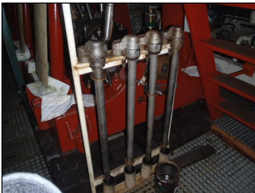
Burner rack containing mechanical and atomizing steam barrels
